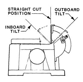
CHAMFERING is removing only the corner of the edge of a board. Normally a chamfer is made with one cut; therefore, a cut deeper than 1/16" may be made.
